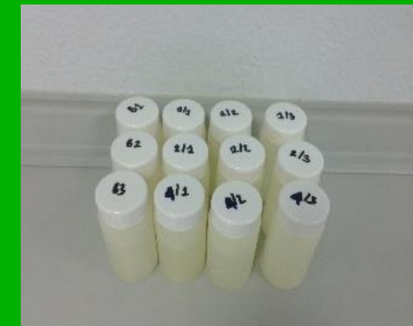
The samples in vials for Cherenkov counting
