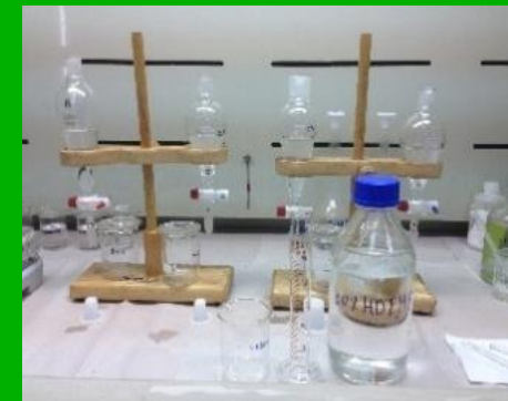
Liquid extraction using 10% HDEHP in toluene
