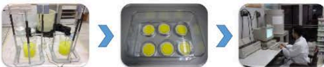
Figure 3 Seawater Preparation for 137 Cs measurement using AMP technique and gamma spectrometry
