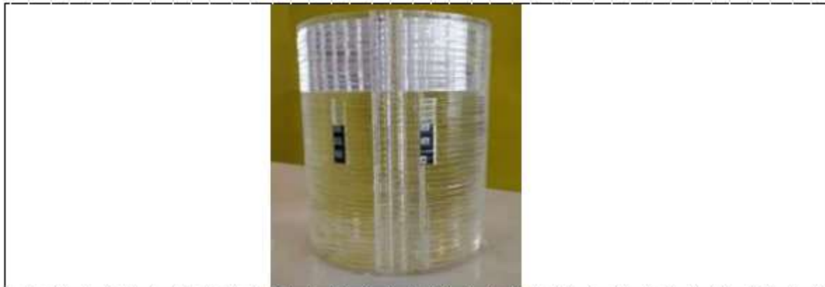
Figure 2. The nanoDot dosimeters were placed in the cylindrical phantom at the depth of 3 mm.
