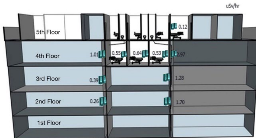
Figure 3. Placement of OSL plates used to measure radiation on the 5 th floor.
