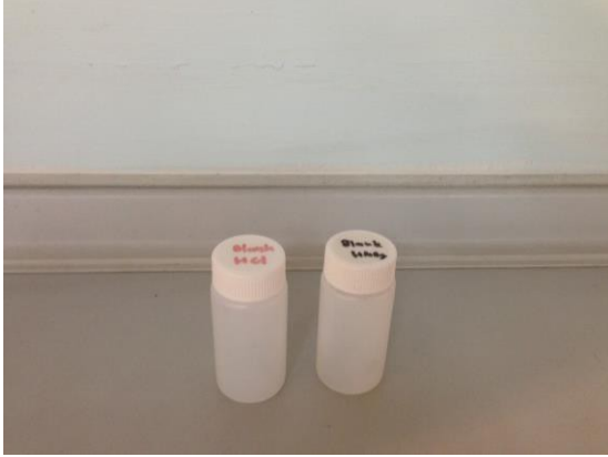
Figure 1. Blank samples of the 16 mL of 0.1 M HCl and 1 M \text{HNO}_3 in polyethylene vials.
