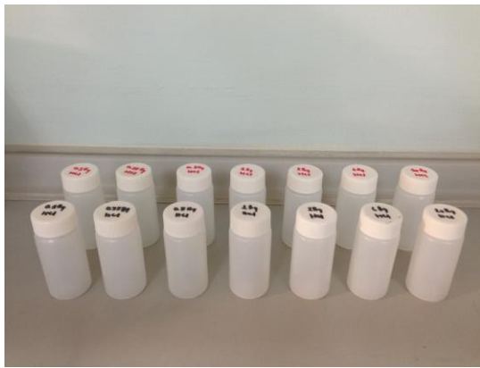
Figure 2. Series of ^{90}\text{Sr}/^{90}\text{Y} prepared solution sources of the 16 mL of 0.1 M HCl and 1 M \text{HNO}_3 in polyethylene vials.
