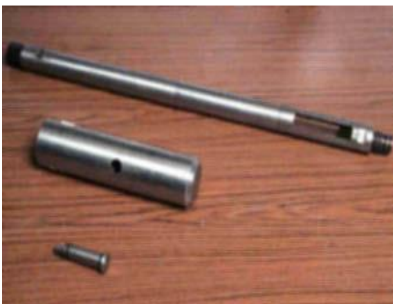
Gauge for measuring the density of well fluids
