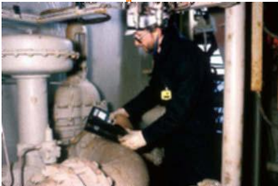
Monitoring the outside of plant and equipment using a dose rate meter (courtesy: National Radiological Protection Board, UK) (ภาพจาก Safety Reports Series No. 34, IAEA, Vienna (2003))
